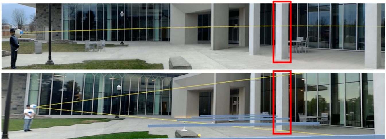
Figure 1: Gaze ray visualizations in AR. Top: the single ray without occlusion cues is visually ambiguous. Bottom: The double ray and parallel bars are designed to reduce visual and spatial ambiguity. We add the red highlight to indicate the target column for the readers, but note that this is not visible to the AR viewer.
