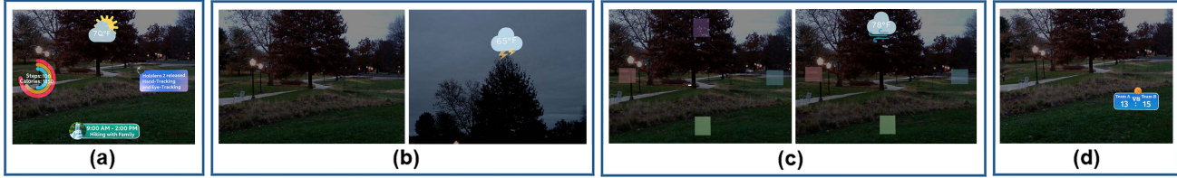
Figure 2: AR implementations of: (a) eye-glance interface; (b) head-glance interface, in which user looks up at the sky to acquire information about the weather; (c) gaze-summon interface, in which user gazes at the top visual target to acquire information about the weather; and (d) virtual basketball scoreboard used in our experiment’s monitoring task.
