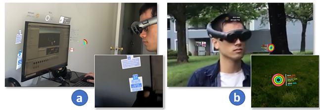
Figure 2: Two scenes from the video prototype: (a) stationary use case in which all widgets are located at the edge of a physical monitor; (b) follow mode with head glance (HG) interface in which the fitness, weather and music widgets follow the user and stay outside the periphery.
