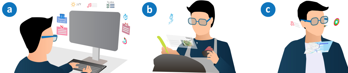
Figure 1: Using Glanceable AR interface in three everyday scenarios: (a) working in front of a desktop computer with glanceable widgets residing at the edge of the physical monitor; (b) cooking with recipe and timer widgets following the user for hands-free access of information; (c) walking outside with music, fitness and map widgets following the user; a notification notifies the user about accomplishing the daily step goal.
